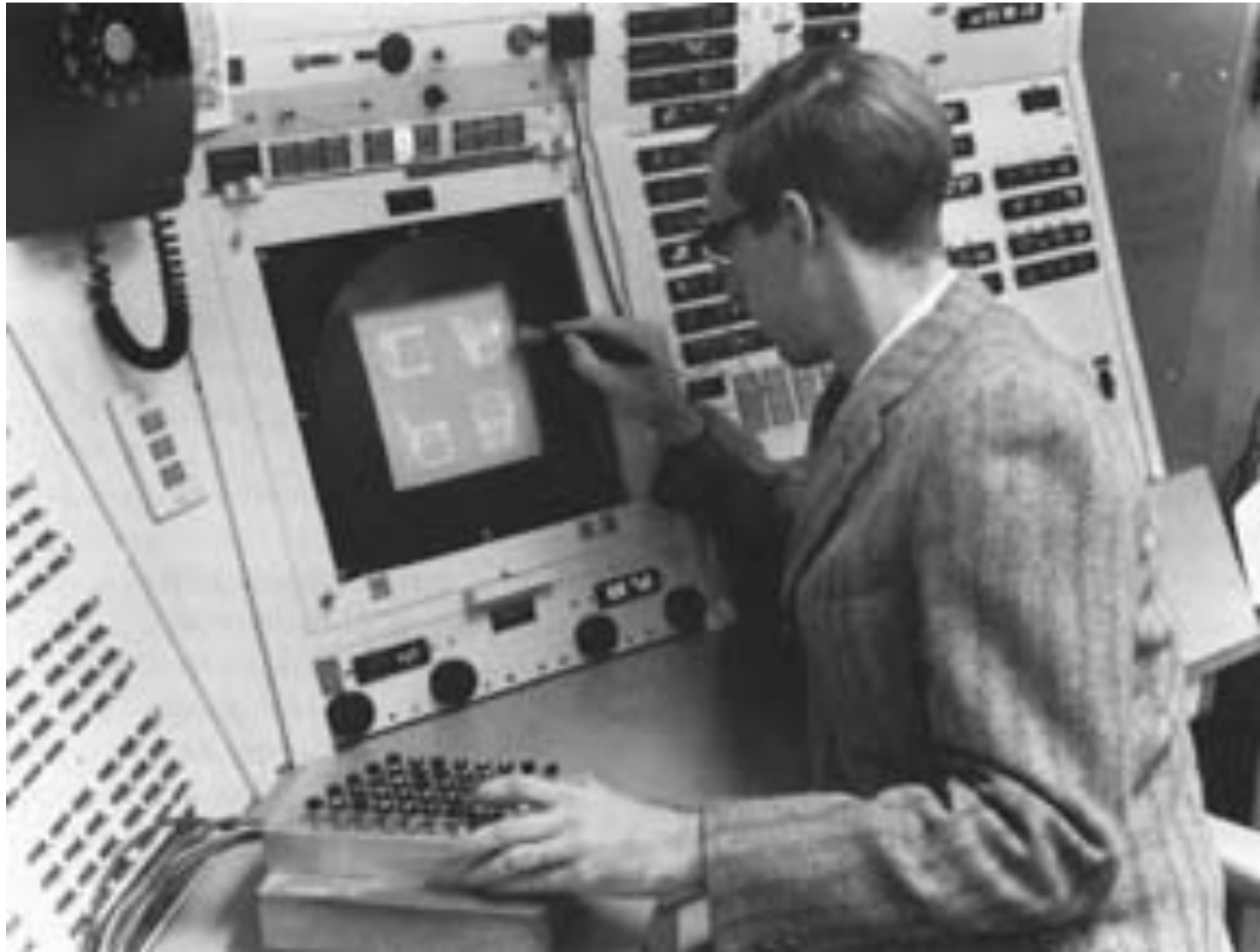
Ivan Sutherland demonstrating the Sketchpad system on the console of the TX-2 at MIT(1963)
